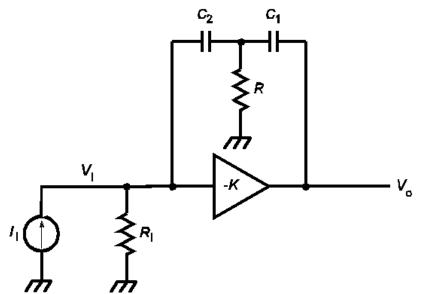
The design equations of Part 1 constrained the damping ratio,  $\zeta$ , of the pole-pair to unity. ( $\zeta = \cos(\phi)$ , where  $\phi$  is the quadratic pole angle.) A useful design parameter, the pole-zero separation, will be given its own symbol as defined:
