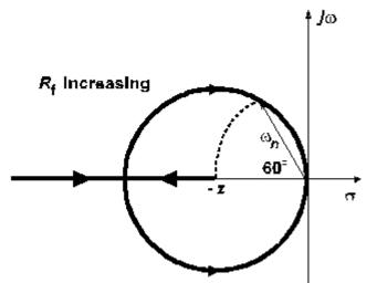
At a pole-zero separation of zero, a 60° pole angle results, which establishes the minimum frequency peaking,  $M_m$  as 1.15 (or 1.25 dB) and minimum pulse overshoot fraction,  $M_p$  as 16 %. For a somewhat useful compensator with one octave of pole-zero separation,  $\gamma = 2$ , and  $\zeta = 0.25$  ( $\phi = 76^\circ$ ),  $M_m = 2.97$  (or 6.3 dB), and  $M_p = 44$  %.
